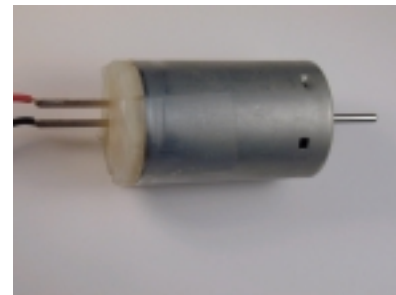
Fig 3. 12V DC Motor used for comparisons.
