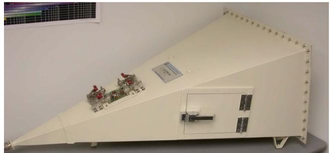
**Figure 19 - Small GTEM Cell with IC Test Board Port**
